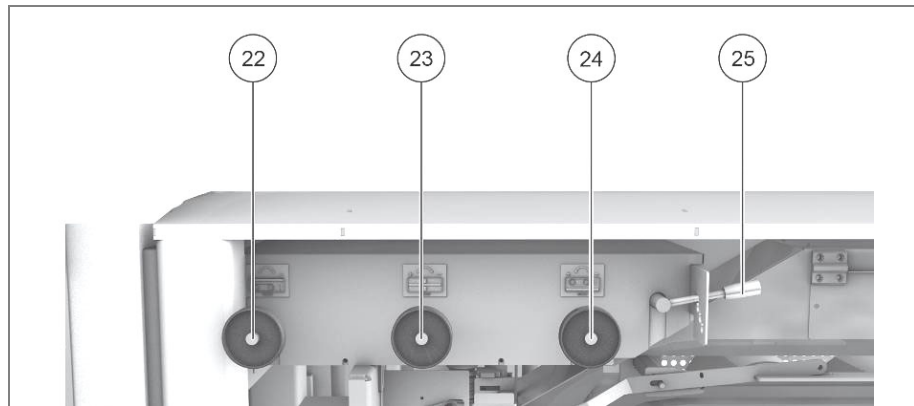
Abb. 4: Control elements of hand wheels (front side SBM-M 1000/1500 D2)
